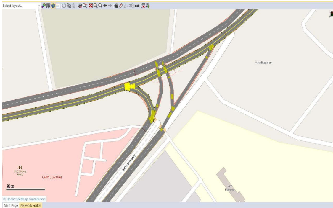
Fig 3: Map from VISSIM Software for Maddilapalem Junction
